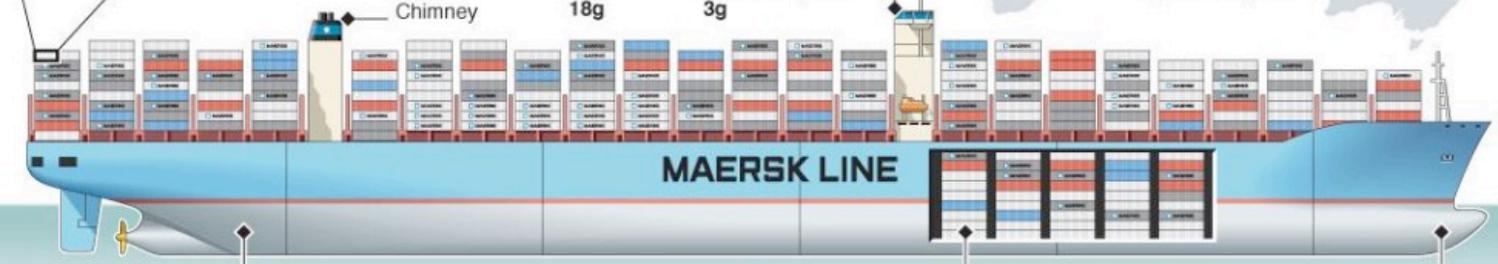
**Propulsion:** Twin 32MW (43,000hp) diesel engines drive two propellers at lower design speed than traditional container vessels – reducing fuel consumption by 37% and CO2 emissions per container by 50%\*
